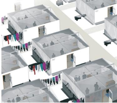
Due to the ability to install hard or soft wall panels, the shelter provides an ideal platform for installation of role-specific equipment. This allows the shelter to be configured for other camp facility solutions such as ablutions, mini-gym and welfare facilities etc. With a further ability to interconnect multiple shelters to form larger complexes, the versatility and potential of these systems is extraordinary.
